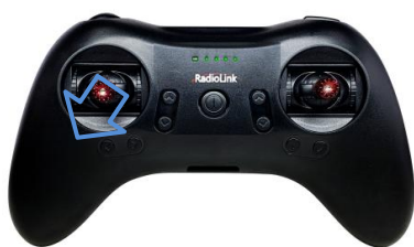
The green LED of F125 off means it is disarmed with success.
