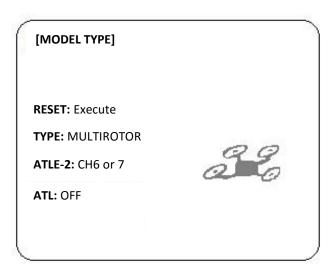
**Note:** For AT9S, the throttle phase needs to be set REV while that of T8FB and AT10II are REV by default.
