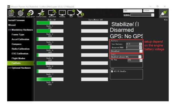
There are different parameters setting such as throttle PWM, battery voltage to enable Mini Pix failsafe function. When the set parameter is reached, eg. If the throttle PWM value or the voltage is lower than the value set, then the failsafe is enabled and the aircraft will take corresponding action such as Return to launch(RTL), Continue to flight and Landing. To ensure the aircraft safety, RTL is normally set as the action following failsafe enabled.
