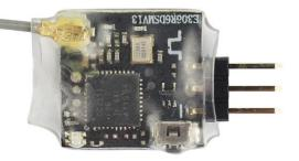
Radiolink R6DSM, 2.4G 10 channels receiver, DSSS and FHSS spread spectrum working synchronously, 1.5 gram weight, SBUS and PPM signal support, use for Radiolink transmitters AT9, AT9S , AT10 and AT10II, is the best choice for racing drone.
