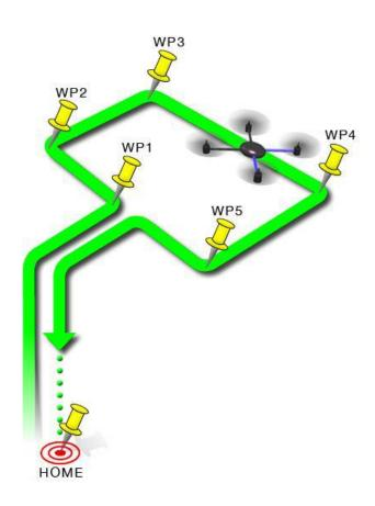
AUTO mode incorporates the altitude control from AltHold mode and position control from Loiter mode and should not be attempted before these modes are flying well. All the same requirements apply including ensuring that vibration levels and compass interference levels are acceptable and that the GPS is functioning well including returning an HDOP of under 2.0.
