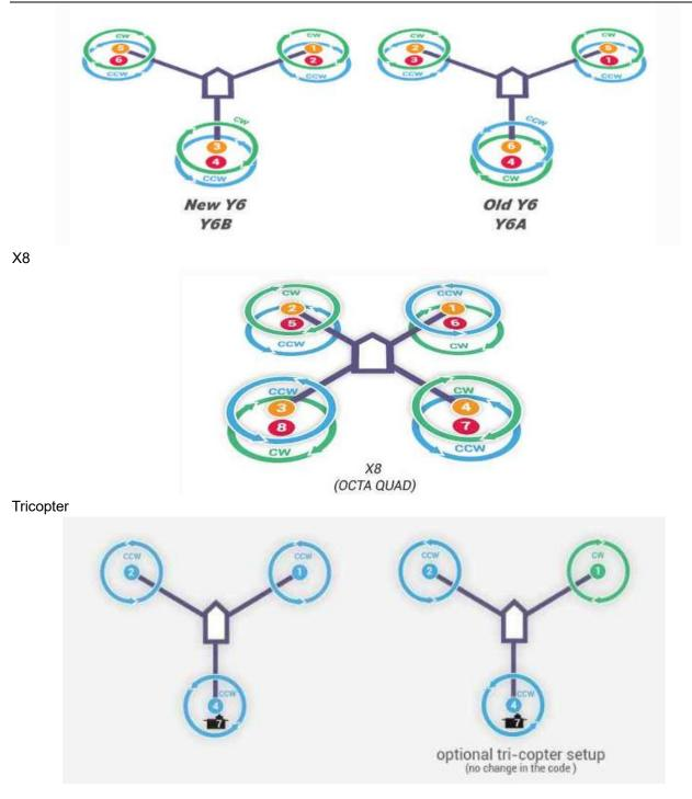
**Note** Since there's no voltage output from the flight controller, an extra BEC module needs to be connected to power supply servo for this model frame
