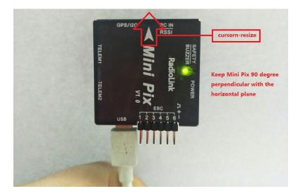
6. Place vehicle on its BACK and press any key to save setting.
