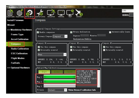
Please fixed Mini Pix and TS100, then click "Start" and turn Mini Pix and TS100 till the progress bar of Mag 1 and 2 to the end and comes out the MAG\_CAL\_SUCCESS marked words.
