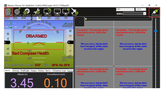
Under Initial Setup--Mandatory Hardware--select Accel Calibration from the left-side menu--Click Calibrate Level to start the calibration.
