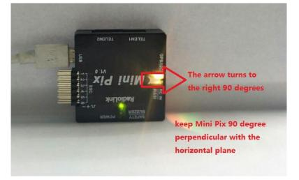
4. Place vehicle DOWN and press any key to save setting.
