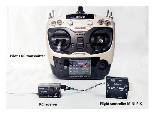
Make sure transmitter and receiver connect success and work with SBUS signal.
