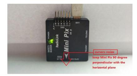
5. Place vehicle UP and press any key to save setting.
