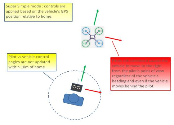
Super Simple mode is the same as simple mode except that it uses the vehicle's position relative to home instead of the vehicle's initial heading when it was armed. This means that no matter where the vehicle is, pulling the pitch back will cause it to return towards home regardless of the vehicle's actual heading.
