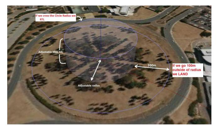
If the vehicle strays outside these borders it will switch into RTL or LAND. At the moment the fence is breached a backup fence is erected 20m further out (or up). If the copter breaches this backup fence (for example if the vehicle is not set up correctly or the operator takes control but is unable to bring the copter back towards home) the copter will be switched into RTL again (and another backup fence an additional 20m further out will be created).
