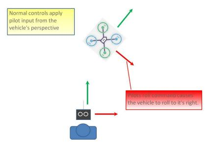
Without Simple or Super Simple enabled, the pilot's transmitter stick inputs are applied in the orientation of the copter. For example, in the diagram above when the pilot applies roll input right (red) the vehicle rolls to its right.
