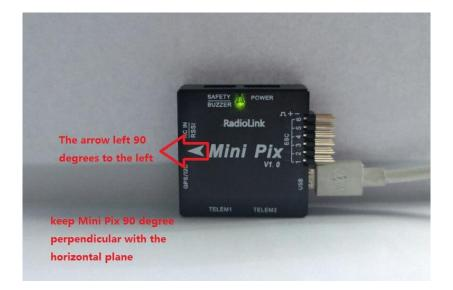
3. Place vehicle on its RIGHT side and press any key to save setting.
