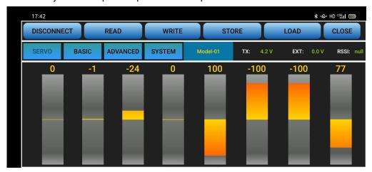
(DIS)CONNECT: When APP is opened on the mobile and T8FB is powered on, click CONNECT and a list of Bluetooth devices will pop out and select the RadioLink device to make connection. The red and green leds will flash with DD sounds, press any of the trimmer buttons of T8FB to stop the DD sounds and the servo range will display on the APP. If fails, press DISCONNECT and CONNECT again.
