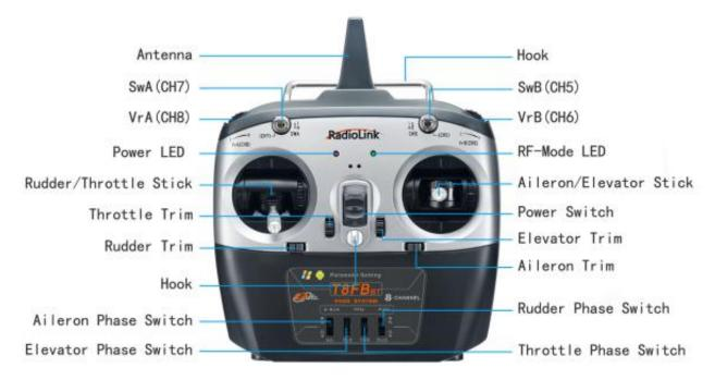
**Note** The phases of the 4 channels can be easily changed by prodding the corresponding phase switches instead of modifying the parameter data in the software/APP.
