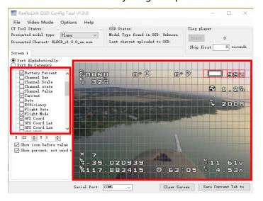
When complete the setting, click File on the left top and click "Save OSD file" to save the set parameters. Next time when the same param. needed, click File and "Open OSD File" to directly reach the personalized data.
