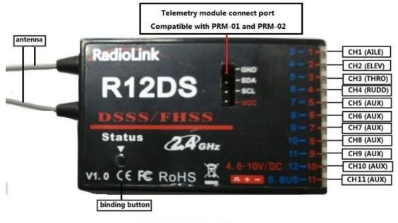
PWM signal working mode: Red LED, output 11 channels PWM signal
