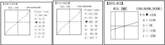
Note: The throttle and pitch curves for the normal condition is always on. They cannot be inhibited. The other four conditions are activated with their throttle curves or throttle hold.
