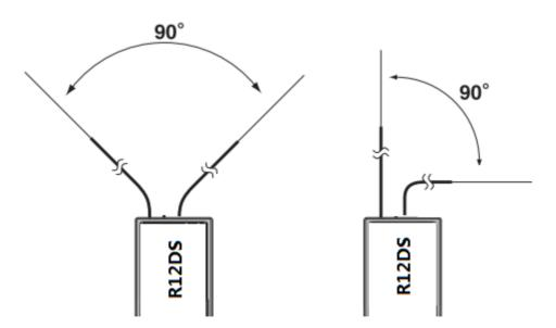
② Big models may contain metal parts that influence signal emission. In this case, antennas should be positioned at both sides of the model to ensure the best signal status in all circumstances.
