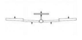
BUTTERFLY simultaneously moves the flaps, twin ailerons and elevator, and is usually used to make steep descents or to limit increases in airspeed in dives. Separate two BUTTERFLY settings are available. (CRI1/CRI2)
