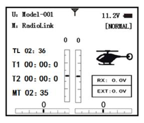
Find telemetry information: under BASIC MENU, select RECEIVE, presses PUSH to enter, you can find the telemetry info, shown as below. RX is receiver voltage, EXT is external voltage. Also temperature and engine speed (EXT, TEMPERATURE, RPM, and GPS all need telemetry sensor). RSSI is signal strength, NULL is for no signal, and 0 is for max.
