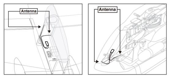
③ Antennas should be kept away from metal conductor and carbon fiber at least half inch away and no over bending.
