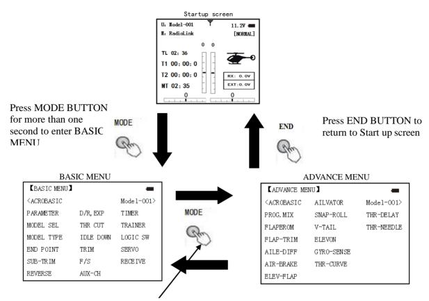
Press MODE BUTTON to switch between BASIC and ADVANCE MENU
