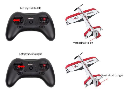
In manual mode, operate the joystick of the transmitter. If the movement of the control surface of the corresponding channel is reversed, enter the setting page of the transmitter to adjust the transmitter phase of the corresponding channel.
