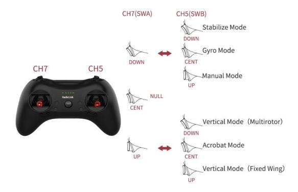
\*When using the T8FB transmitter, the flight modes are switched by CH5(a 3-way switch) and CH7(a 2-way switch) by default. The definition of the flight mode switchover switches is as the picture below:
