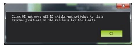
Joysticks can be calibrated as following , both (Ch1 to Ch4) are pushed to the limits(up/down/left/right) **Note:** AT9S/AT10II/AT9/AT10 can be calibrated as the below example T8FB
