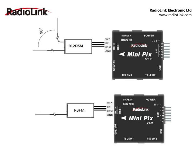
Binding the transmitter to the receiver is essential. Otherwise, the aircraft cannot take off. RadioLink receivers R12DSM/R6DSM are compatible with transmitters AT9/AT9S/AT10/AT10II while R8FM is compatible with transmitter T8FB.
