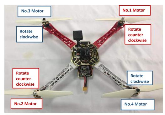
Note: Never install the props before finishing setting parameters of aircraft to ensure the safety.
