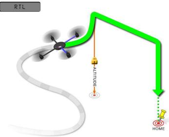
RTL Mode works with GPS, which is indispensable to locate before changing to this Mode. The Mode commands the aircraft to return "HOME" where it takes off. Therefore, "HOME" should always be the place that the GPS locates where the aircraft actually takes off, without obstacles and far away from crowds.
